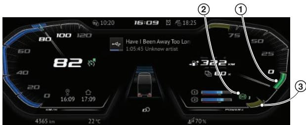
The available power can be limited by certain conditions. Battery State of Charge, temperature, and the motor temperature may trigger the limitation, at which point yellow blocks will be visible in the Digital Instrument Panel. This yellow visual overlay (3) represents the amount of power not available. The green bar (1) shows the amount of energy that is currently being recuperated (braking power). The green telltale (2) shows the activation and, if applicable, regenerative braking power level.
